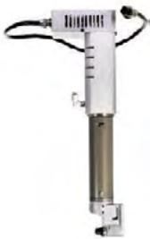
The circular knife positions the material using high-speed rotating blades driven by a servo motor. The tool can be equipped with circular blades, decagonal blades, among others. These are especially suitable for cutting woven materials.
