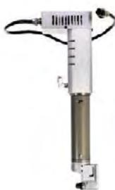
The circular knife positions the material using high-speed rotating blades driven by a servo motor. The tool can be equipped with circular blades, decagonal blades, among others. These are especially suitable for cutting woven materials.
