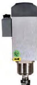
With an imported spindle, it has a rotation speed of 24,000 rpm. It is used for cutting hard materials with a maximum thickness of 20 mm. The customized cleaning device removes production dust and debris. The air cooling system extends the life of the blade.
