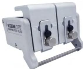
The Evolution3 Double Graphik tool head comes as standard and has two individual blade holders for two-way cutting. The blades are stronger and more stable than regular blades making the Double Graphik tool ideal for vinyl, banner, cardboard, PVC foamboard up to 13mm (1/2"), foam-centred board, corrugated plastic, paper, pop-up and roll-up materials.
