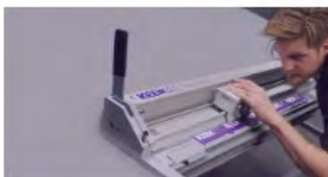
The self-adjusting track roller system fitted to the QuikSwap tool heads provides a strong and smooth movement up and down the length of the cutter bar, with zero sideways movement to ensure a perfect straight line. This, coupled with rigid blade clamping gives perfect blade control and spot-on accuracy, so less wastage and mistakes. On the FreeHand, the underside of the cutter bar has two silicone strips that will grip to the material surface preventing any chance of it slipping.
