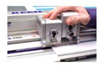
The self-adjusting track roller system fitted to the QuikSwap tool heads provides a strong and smooth movement up and down the length of the cutter bar, with zero sideways movement to ensure a perfect straight line. This, coupled with rigid blade clamping, gives perfect blade control and spot-on accuracy, so less wastage and mistakes.
