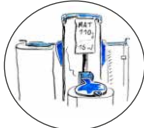
Identification Material identification system on each reel for localisation of the reel
