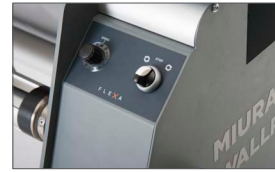
Speed regulator and switch to adjust the rotation of the rewinding shafts
