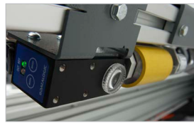
Advanced cutting mark reader
